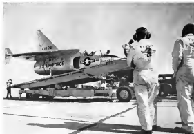
TRAILER BED lowers to horizontal position (above) to pilot on and from the Vertigo. Raising and lowering mechanism is hydraulic.
